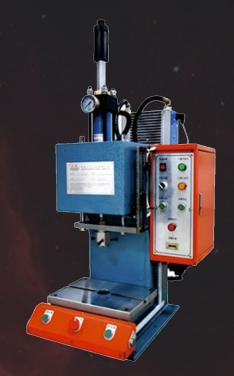
Driven by oil pressure, flexible control, stable running speed, stable pressure, large output adjustment range;
